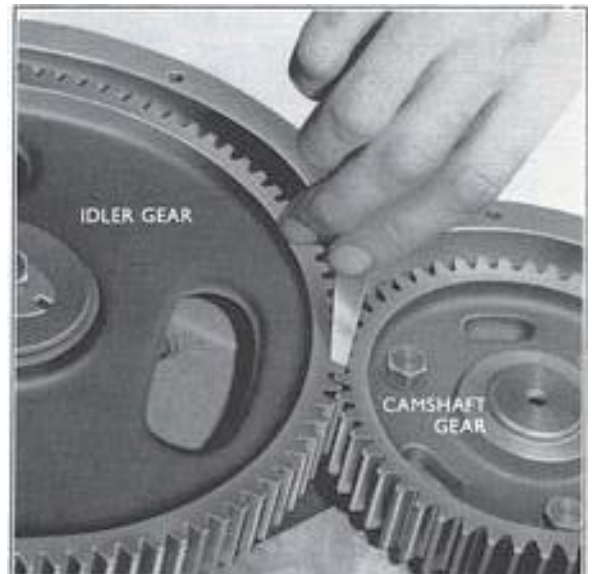
Fig. 9 Checking Timing Gear Backlash
