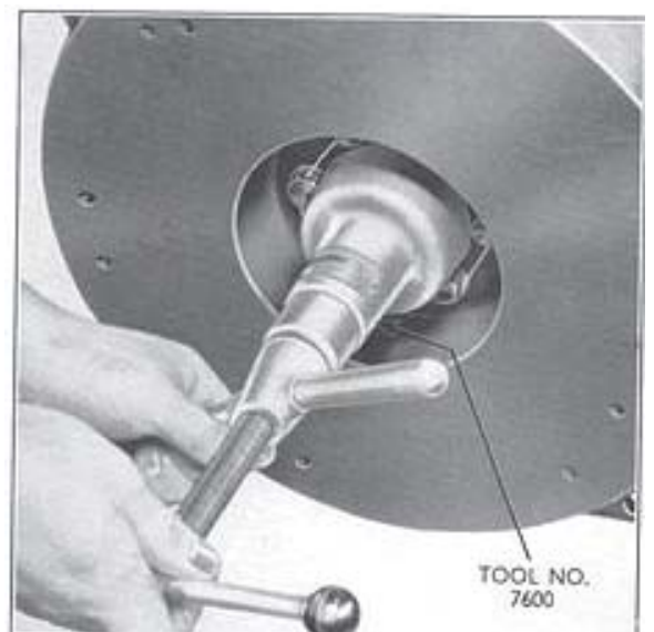
Fig. 19 Removing Clutch Pilot Bearing
